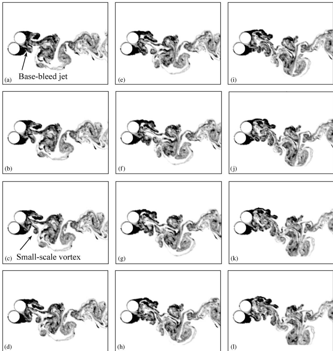
Fig. 5. Numerical flow visualization plots (streaklines) for a “base-bleed” flow regime with P/D = 1.06 , \alpha = 60^\circ , Re = 800 . Equal time-intervals of t^* \equiv tU/D = 0.2 between consecutive plots (a)–(l).
